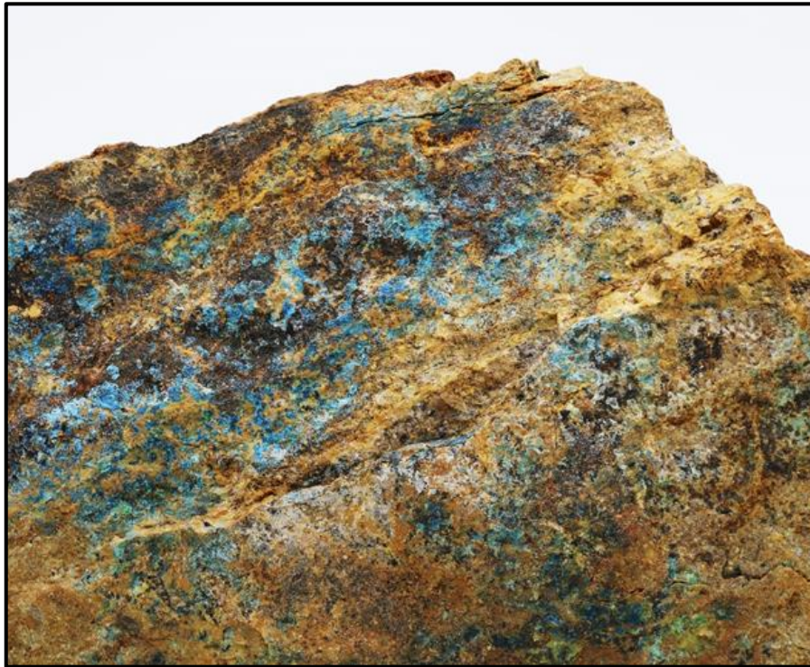
Figure 1: Silicified rhyolite with numerous quartz and carbonate veinlets; Malachite and azurite mineralization. (Rock sample D00227638: 0.4% copper, 29.0 g/t silver)
